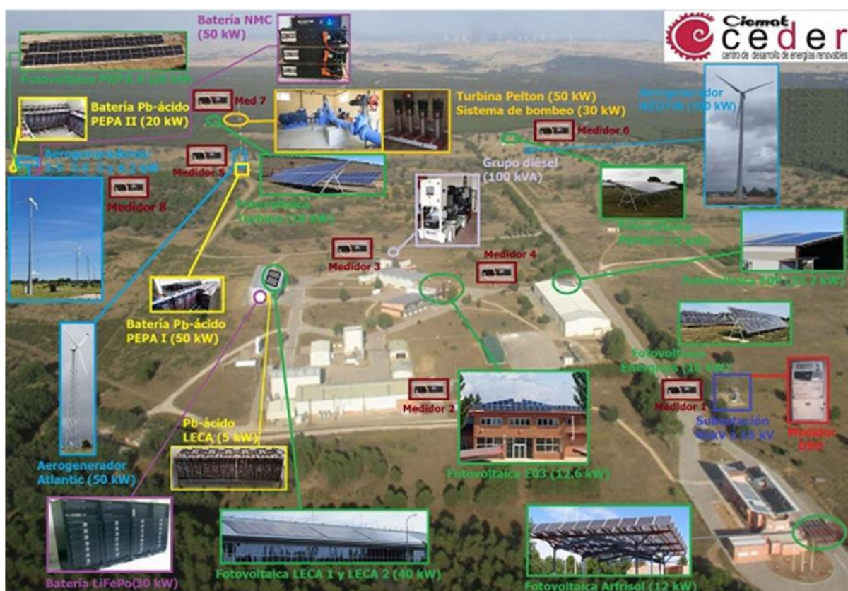
Figure 14: Distribution of the electrical micro-grid elements in the CEDER PED-Lab (Spain). (Source: CEDER-CIEMAT website)
